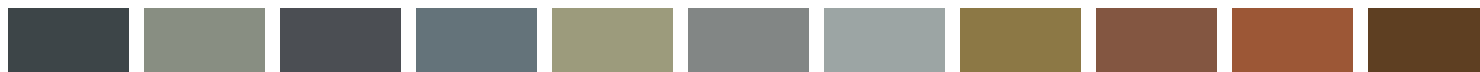
7016 anthracite grey 7023 concrete 7024 graphite 7031 blue grey 7034 yellow grey 7037 dusty grey 7042 traffic grey 8000 green brown 8002 signal brown 8004 copper brown 8011 nut brown
